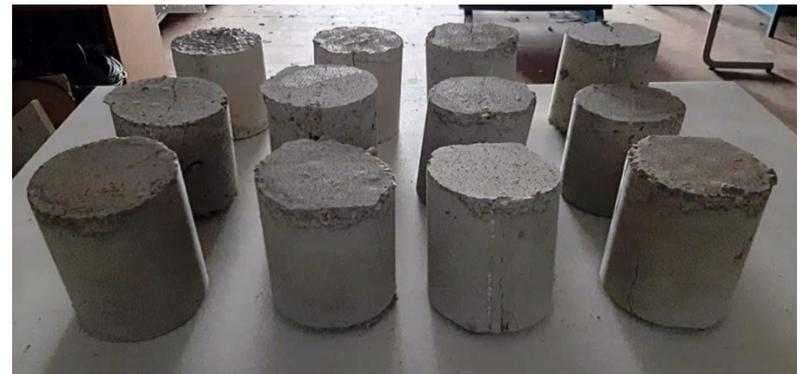
Source : Concrete Blocks Reinforced with *Arundo donax* Natural Fibers with Different Aspect Ratios for Application in Bioarchitecture
